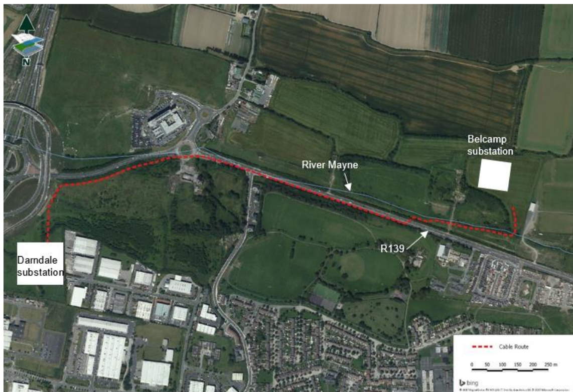
Figure 1.1 Proposed Route of 110kV Underground cable installation
